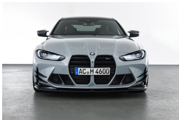
1) Frontsplitter / front splitter
